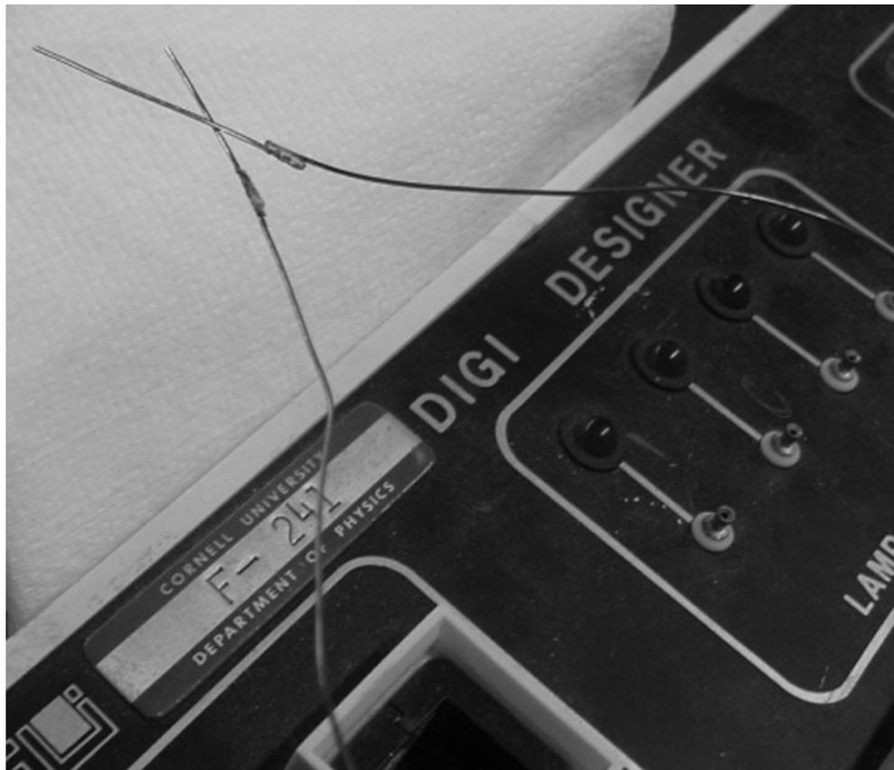
Figure 7: Example of gold wire tips supported on long lever arms.
